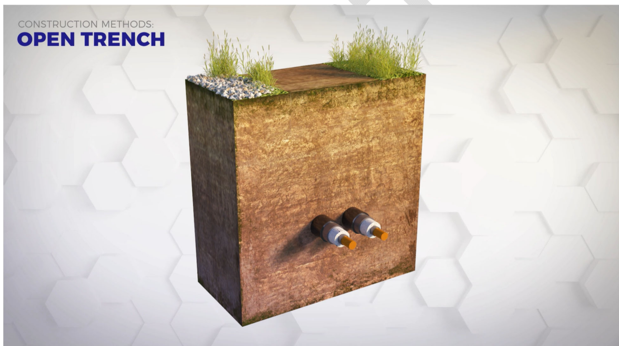
Figure 7-7: Open Trench Approach
