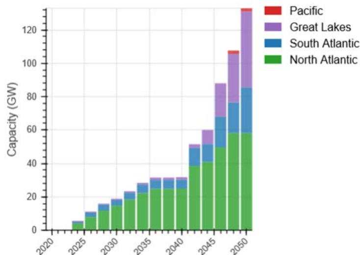
**Figure ES-4. Regional offshore wind energy deployment in a 95% grid decarbonization-by-2050 scenario. Graph reproduced from Mai et al. (2022)**
