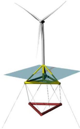
**Figure 17. The TetraSpar substructure concept. Image from Borg et al. (2020)**
