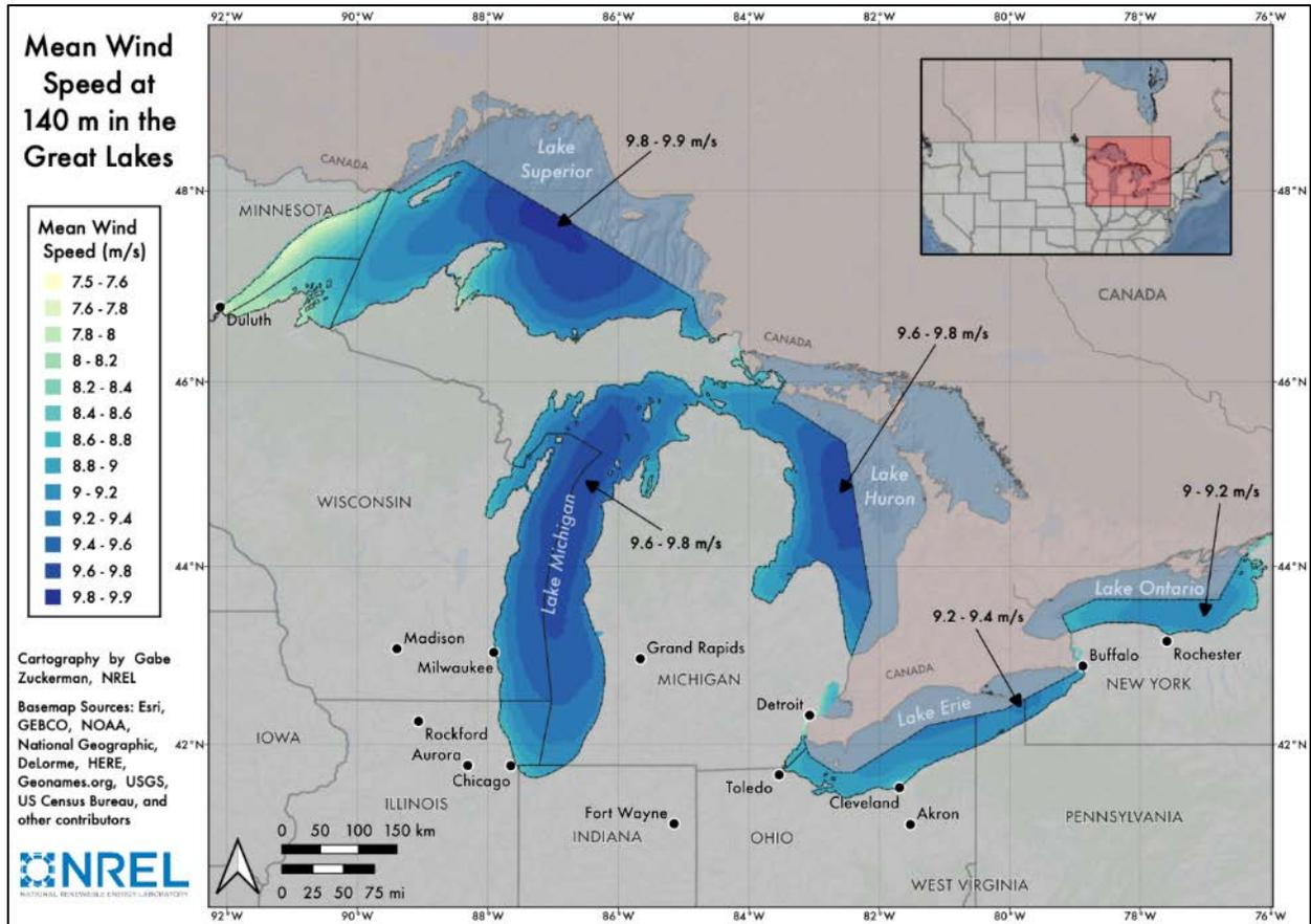
**Figure 4. Mean wind speed at 140 m above water level. Map generated with data from Bodini et al. (2021)**
