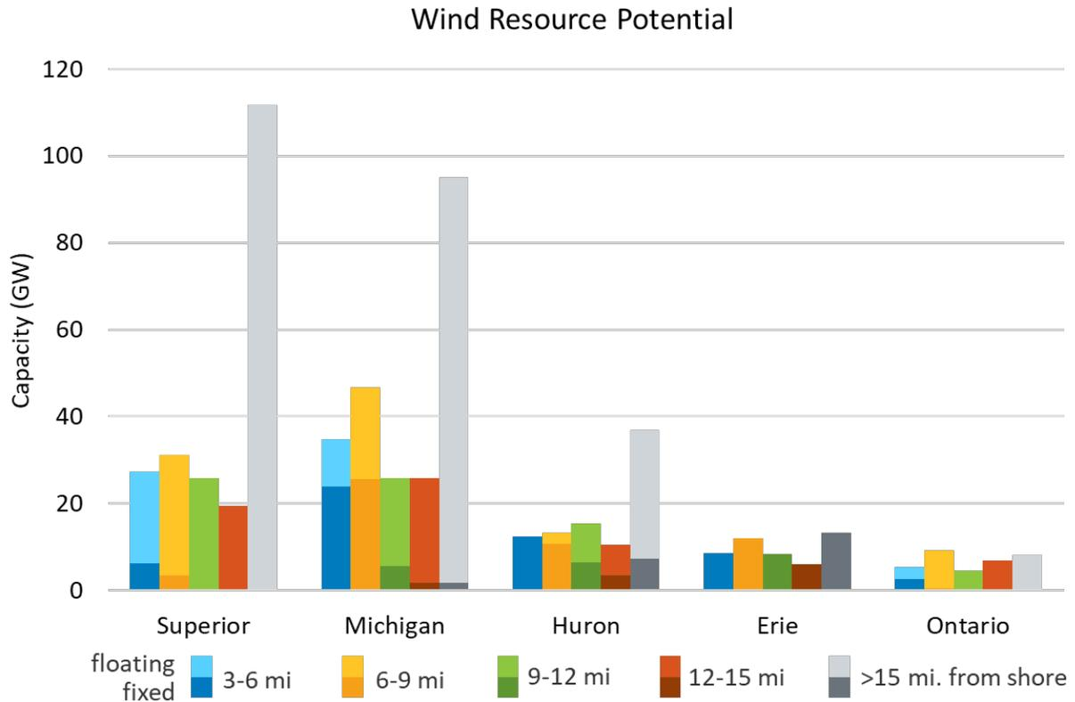
**Figure 33. Great Lakes wind resource potential breakdown by distance to shore, by lake from west to east, and assuming an array density of 5 MW/km<sup>2</sup>**
