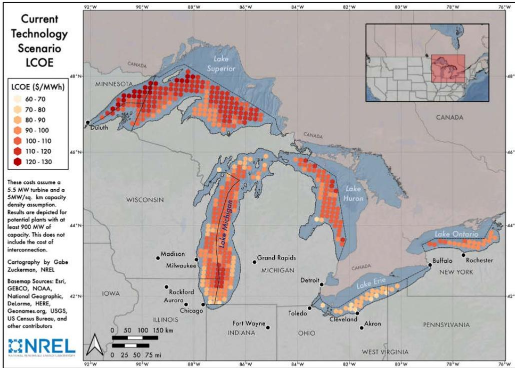
Figure 40. Modeled LCOE in 2035 for the Current Scenario. Map from NREL
