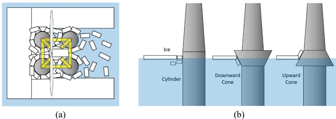
**Figure 14. Nonslender waterline profiles create potential for ice jamming (a), and ice cones induce the bending moment of failure of ice, which exerts smaller loads on the structure (b).
