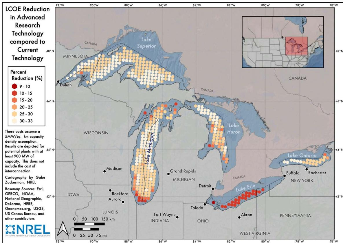
**Figure 42. LCOE reductions when using the Advanced Research Technology Scenario compared to the Current Scenario. Map from NREL**
