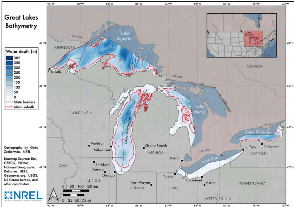
**Figure 6. Water depths in the U.S. Great Lakes shown with the 60-m isobath (nominal depth limit for fixed-bottom offshore wind structures)**
