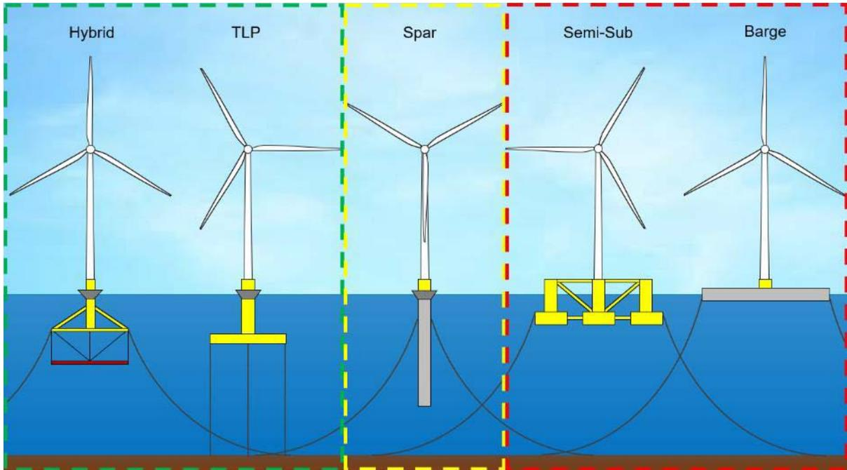
**Figure 16. Common floating substructures that could be used for Great Lakes wind energy (green: most favorable, yellow: less favorable, red: not favorable). Image by NREL**
