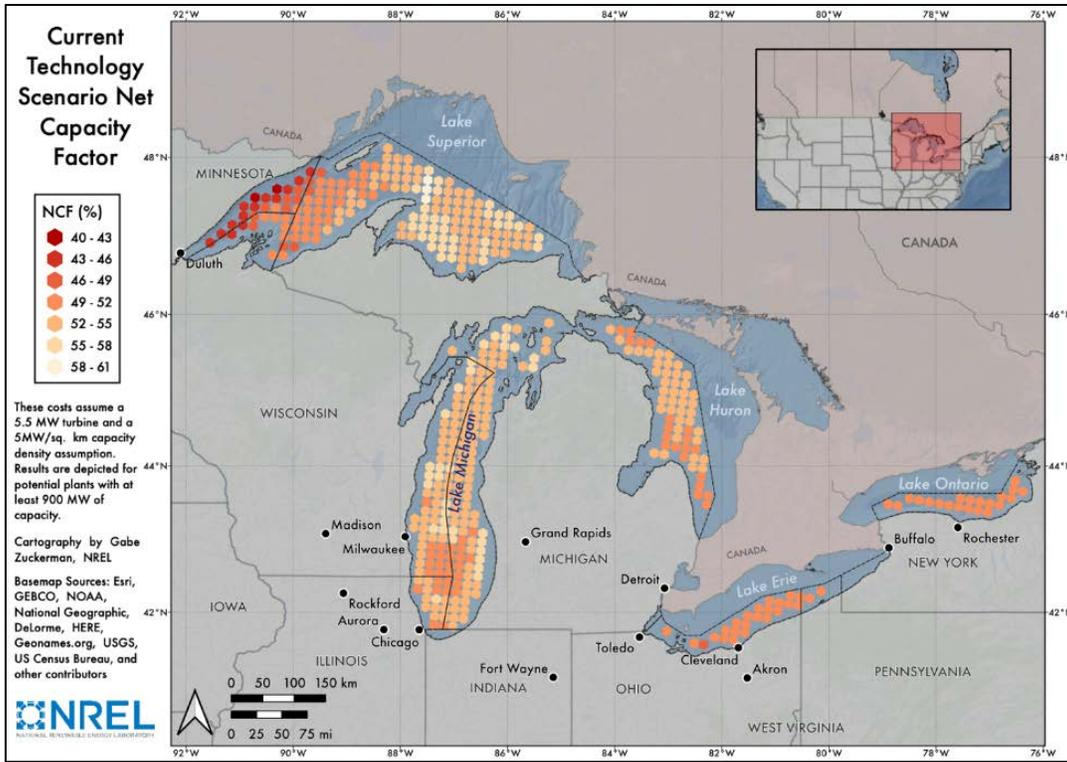
Figure 38. Modeled net capacity factors in 2035 for the Current Scenario. Map from NREL
