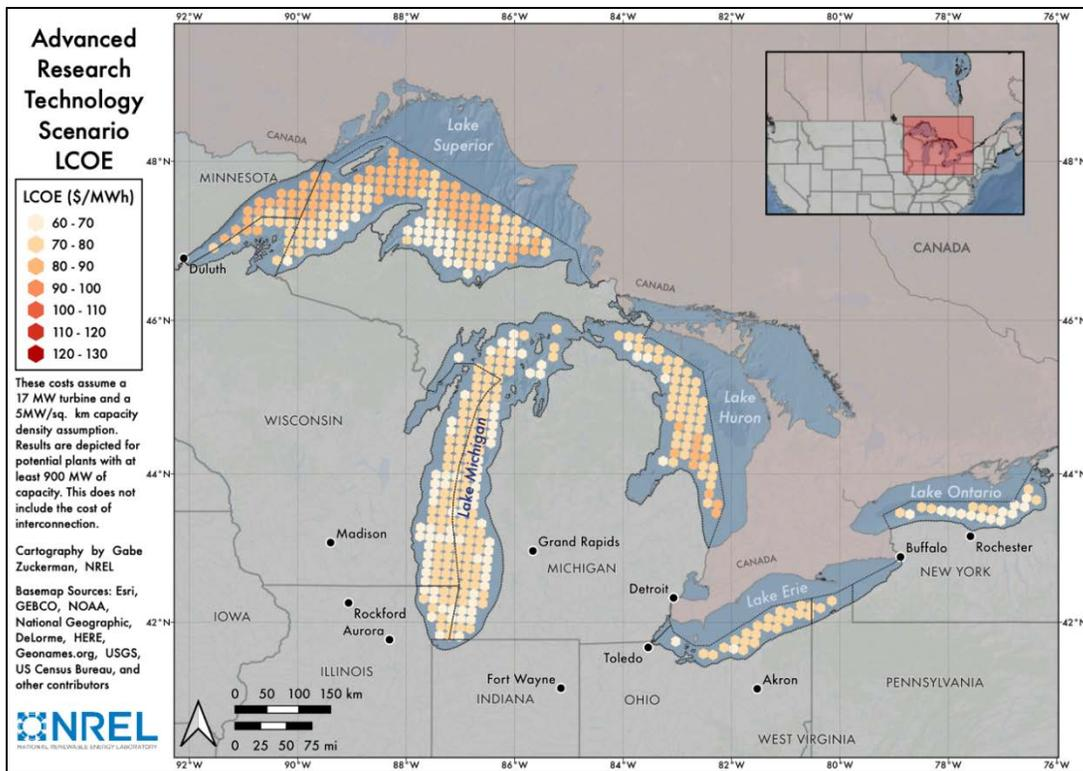
**Figure ES-3. Modeled levelized cost of energy (LCOE) in 2035 for the Advanced Research Technology Scenario**
