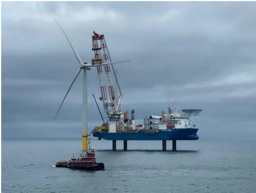
**Figure 9. Example installation vessel used for offshore wind energy development. *Photo by Lyfted Media for Dominion Energy***
