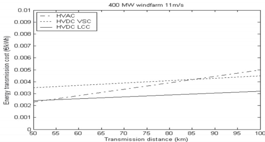
**Figure 23. Energy transmission cost from Figure 22 magnified for 50–100 km. Image from Reed et al. (2013)**
