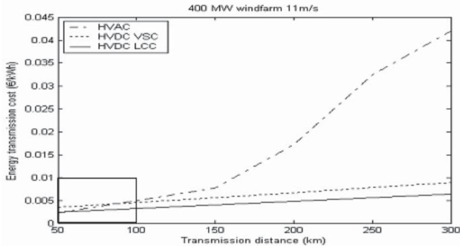
**Figure 22. Energy transmission cost for a 400-MW wind power plant and 11-m/s wind speed for distances between 50 and 300 km. Image from Reed et al. (2013)**
