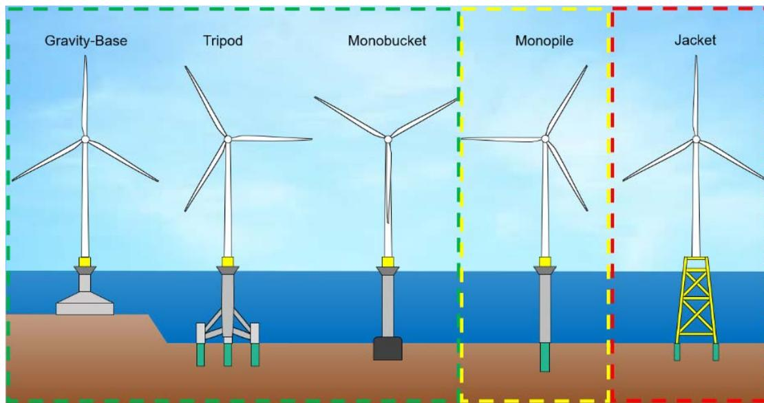
**Figure 15. Possible fixed-bottom substructures for Great Lakes wind energy (green: most favorable, yellow: less favorable, red: not favorable). Image by NREL**
